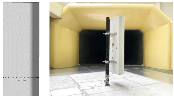
Figure 12 Wind tunnel pressure test of the antenna
